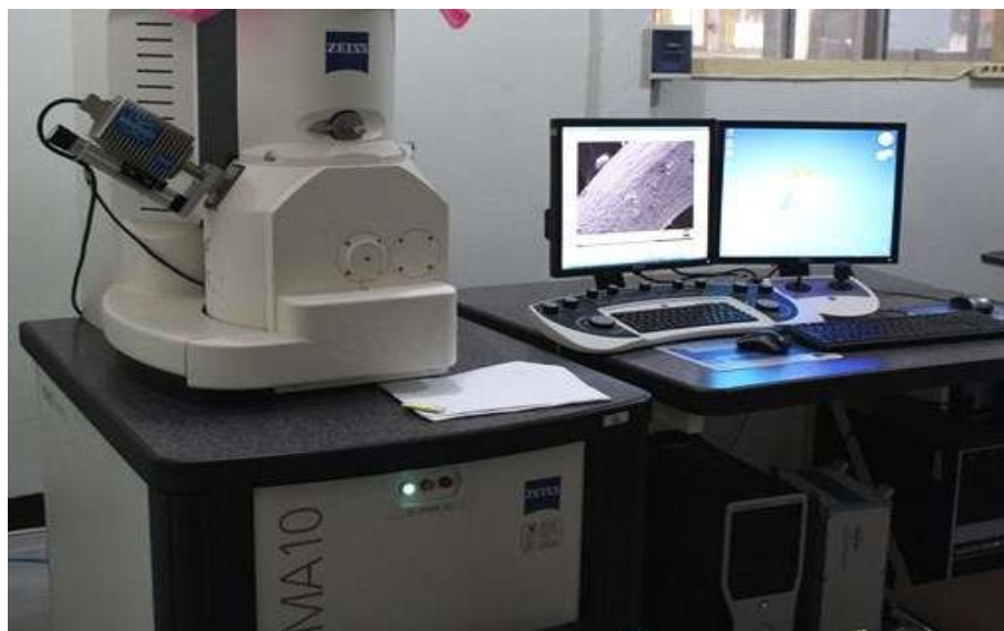
Gambar 16. Scanning Electron Microscope berjenis ZEISS EVO® MA 10.
