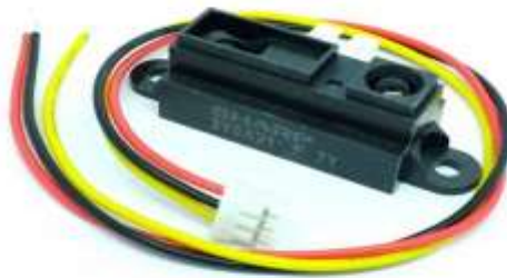
Gambar 2.9. Sensor Infrared SHARP (Sumber : Sheet No.: E4-A00201EN. Date Dec.01.2006 ©SHARP Corporation)
