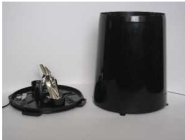
Gambar 3. Alat Penakar Hujan otomatis tipe tipping bucket
