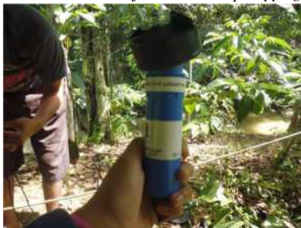
Gambar 3. Alat Penakar Hujan otomatis tipe tipping bucket
