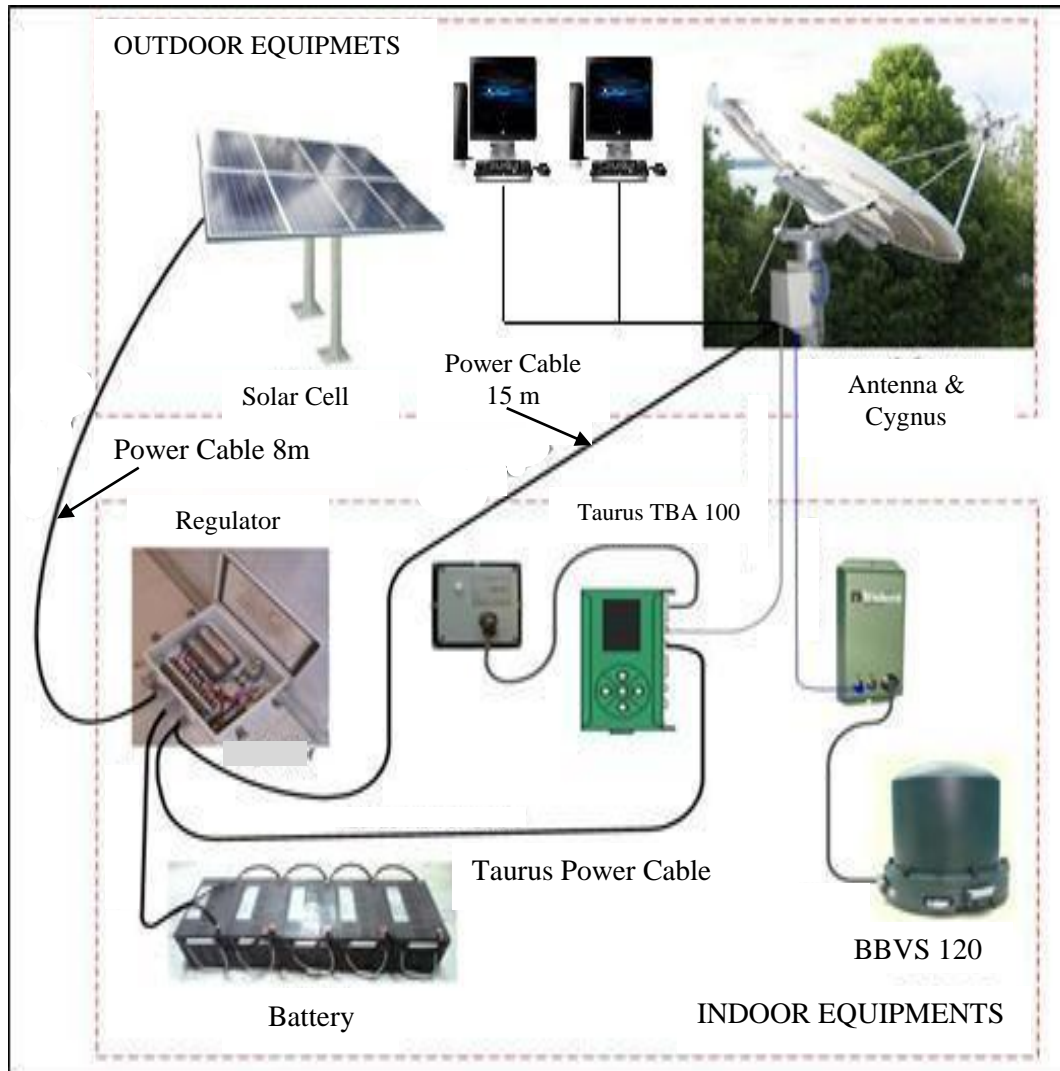
Gambar 6. Alur peralatan accelerograph (Sativa, 2015).
