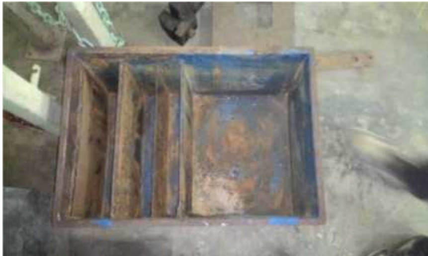
Gambar 3.9 Bak media quenching
