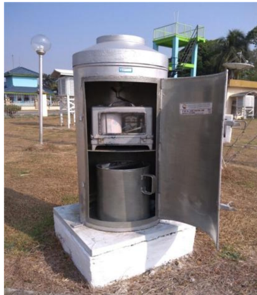
Gambar 4. Penakar hujan otomatis tipping bucket (Sumber: BMKG, 2018)
