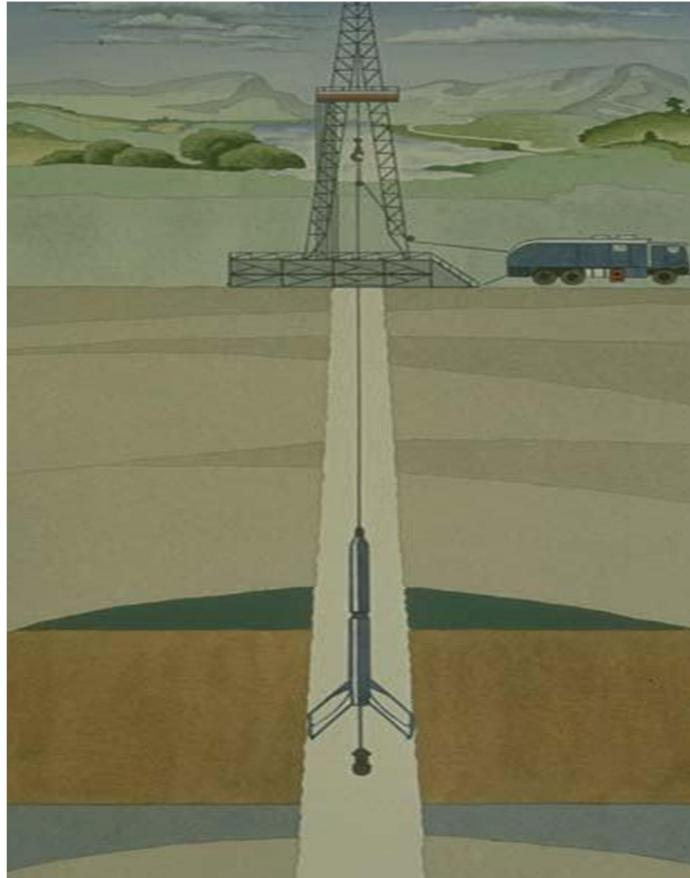
**Gambar 25.** Pengukuran *Wireline Logging* sumur
