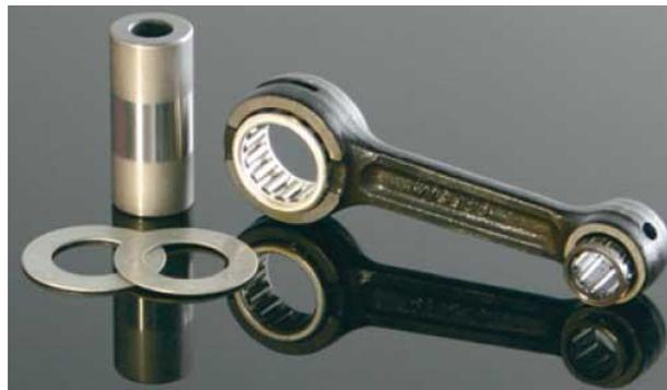
Gambar 15. Batang torak (*Conecting rod*)
