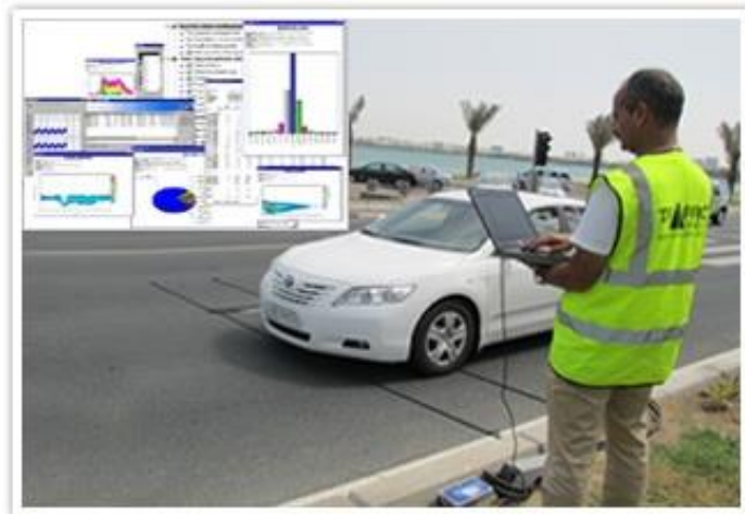
Gambar 10. Alat Automatic Traffic Count
