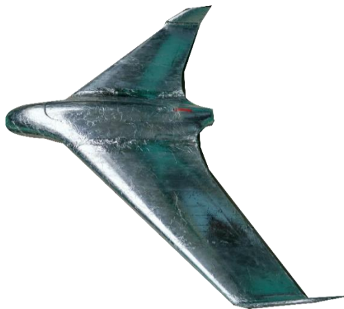
Gambar 2.9 UAV berlapis aluminium foil
