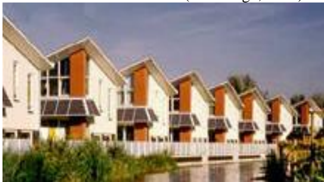
Gambar 2.9. Integral Roof Modules PV (Mintorogo, 2000)
