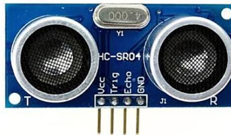
Gambar 2.4 Sensor Ultrasonik HC-SR04
