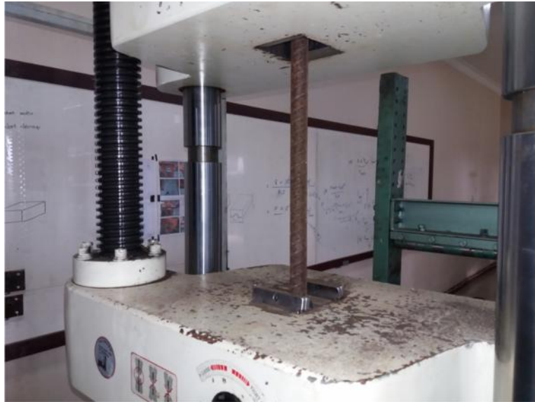
Gambar 3.10. Universal Test Machine (UTM)
