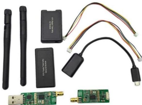
**Gambar 2.9** Modul *telemetry* 433 MHz
