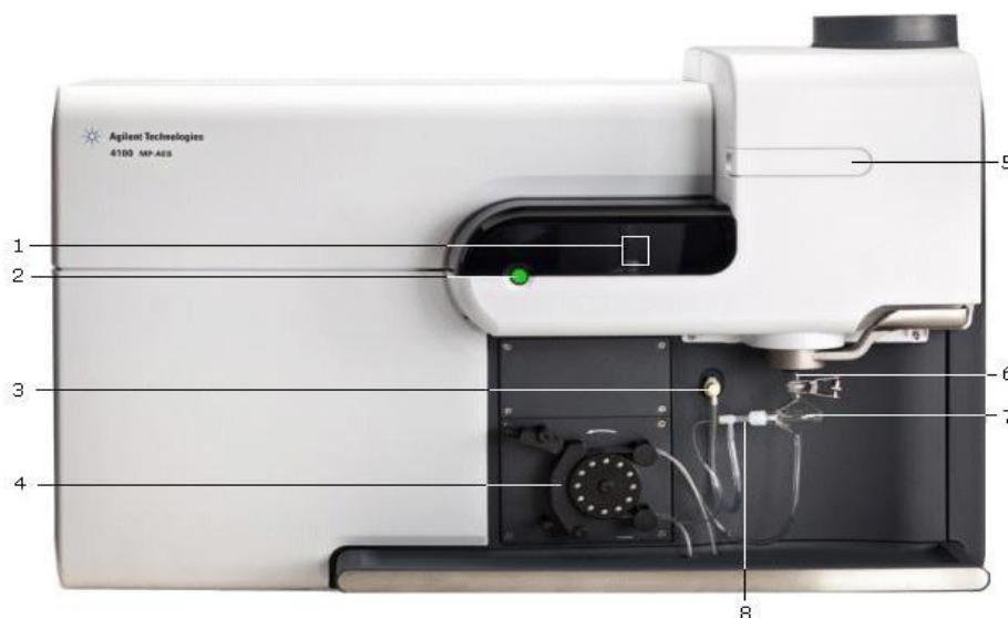
Gambar 8. Perangkat MP-AES Agilent MP-1400 (Keterangan: 1. Plasma viewing window , 2. Plasma enable switch , 3. Nebulizer gas connection , 4. Peristaltic pump , 5. Pre-optic window , 6. Torch , 7. Spray chamber , dan 8. Nebulizer )
