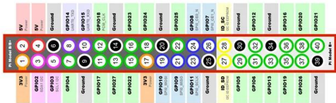
Gambar 2.2 GPIO Raspberry Pi 3 Model B+[5]
