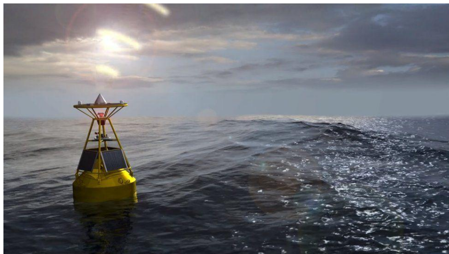
Gambar 2. 3 Merupakan Buoy Tsunami ( https://ichef.bbci.co.uk/news/624/cpsprodpb/3538/production/103642631_buoy2.jpg )
