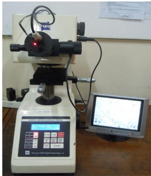
Gambar 26. Alat uji vickers Hardness Tester TH712 Shimadzu
