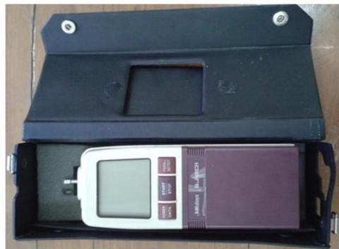
Gambar 11. *Surface roughness taster*
