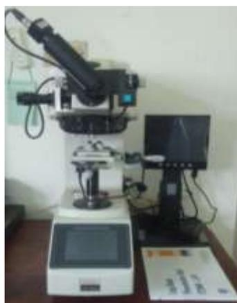
Gambar 24. Alat Uji Kekerasan Vickers (*Vickers Micro Hardness*)
