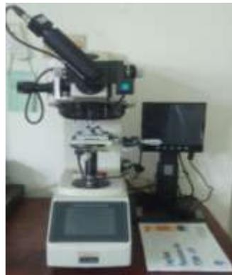
Gambar 9 Alat Uji Kekerasan Mikro Vickers
