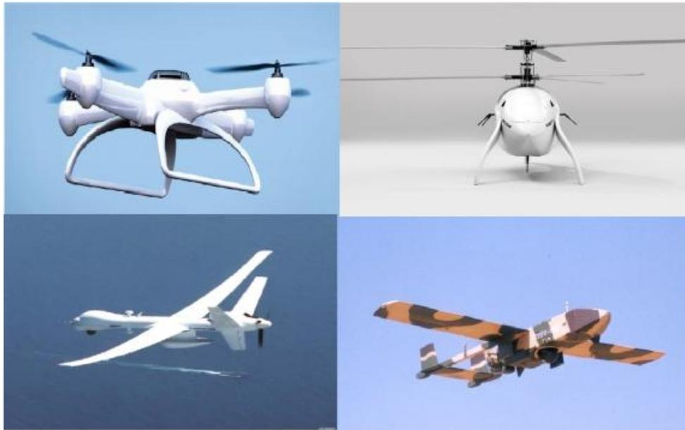
**Gambar 2.4** *Rotary wing* (atas) dan *fixed-wing* (bawah)
