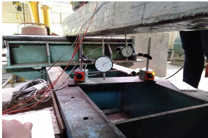
Gambar 4.16 Pemasangan *dial gauge*.
