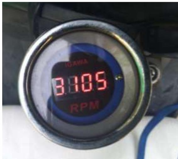
Gambar 9. *Tachometer* digital
