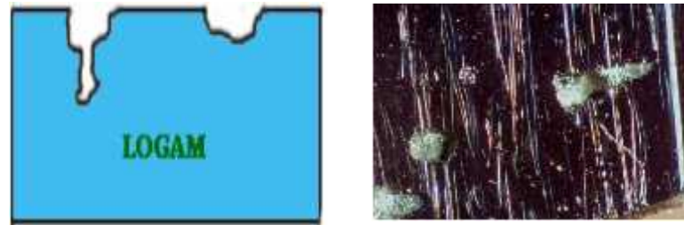
Gambar 2.4. Korosi sumuran ( pitting corrosion ).
