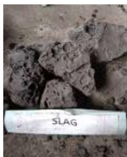
**Gambar 2.** Slag (Sumber: Laboratorium Non-Logam LIPI)
