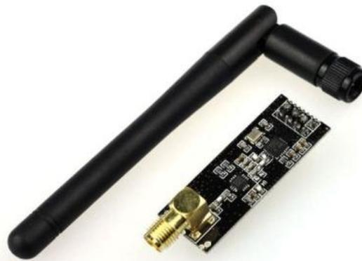
Gambar 2.10. Modul *Transmitter-Receiver* nRF24101+
