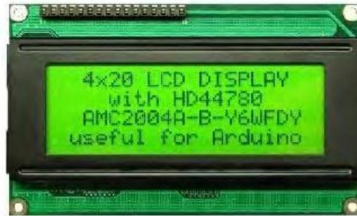
**Gambar 2.15.** *Liquid crystal display (LCD) Character 20x4* (Putro, 2012).
