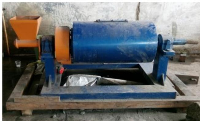
**Gambar 5.** *Ball mill* (Sumber: Laboratorium Non-Logam Balai Penelitian Teknologi Mineral - LIPI).
