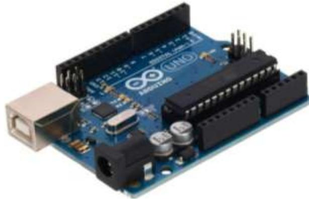
Gambar 2.3 *Board* Arduino Uno
