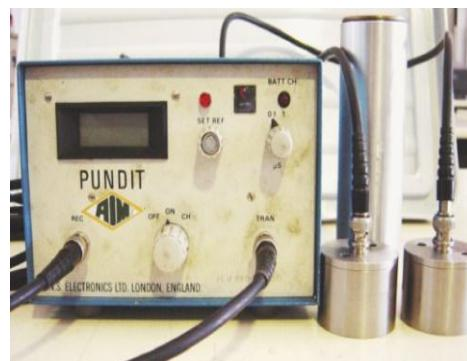
Gambar 5. *Ultrasonic Pulse Velocity* pengujian kuat beton eksisting.
