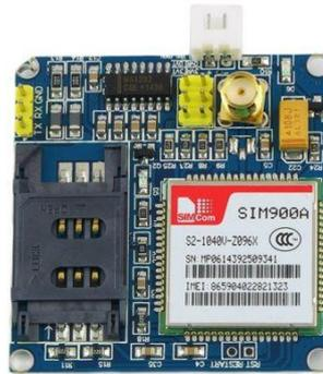
Gambar 2.8 Modul GSM SIM 900A
