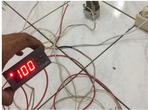
Gambar 3.5 *Thermostat temperature controller*
