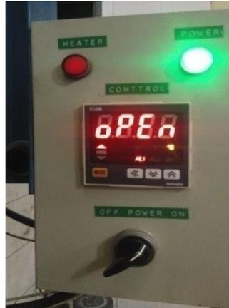
Gambar 14. *Heater Control Unit TC4M*
