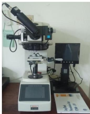
Gambar 23. Alat Uji Kekerasan Vickers (Vickers Micro Hardness)
