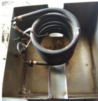
Gambar 16. *Heater Coil*
