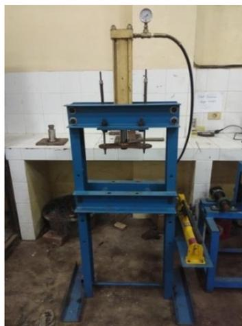
Gambar 12. Mesin Press Hidraulik
