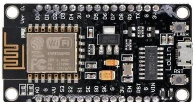
Gambar 3.5 *Board* NodeMCU
