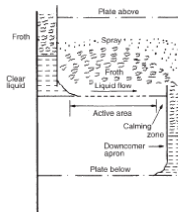
Gambar F.6. Typical crossflow plate (sieve)
