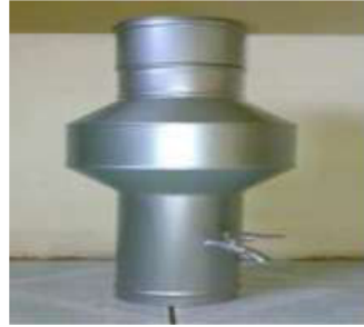
Gambar 2.1 Alat Penakar Hujan Manual Tipe Observatorium
