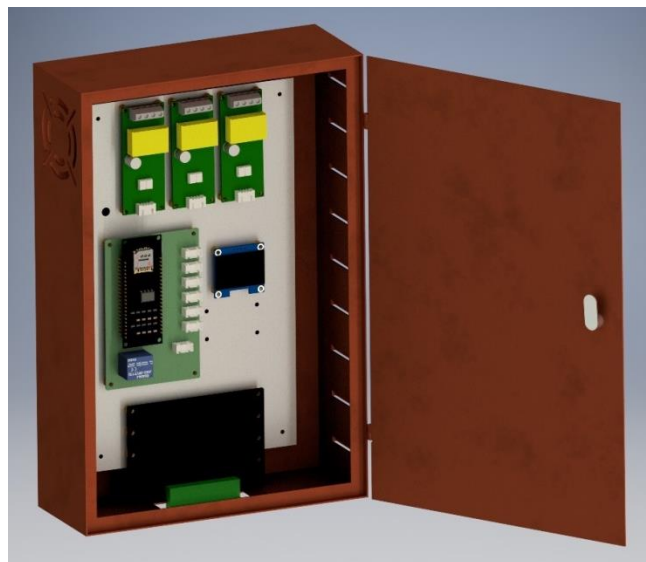
Gambar 2.3 Prototype Monitoring Gardu 3 Phase
