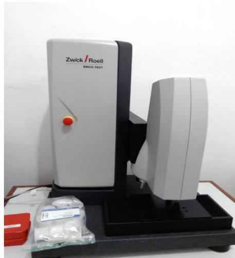
Gambar 38. Alat Uji Kekerasan Vickers (Digital Vickers Micro Hardness)
