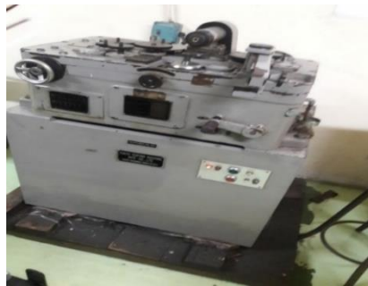
Gambar 3.7. Ogoshi high speed universal wear testing machine type OAT-U
