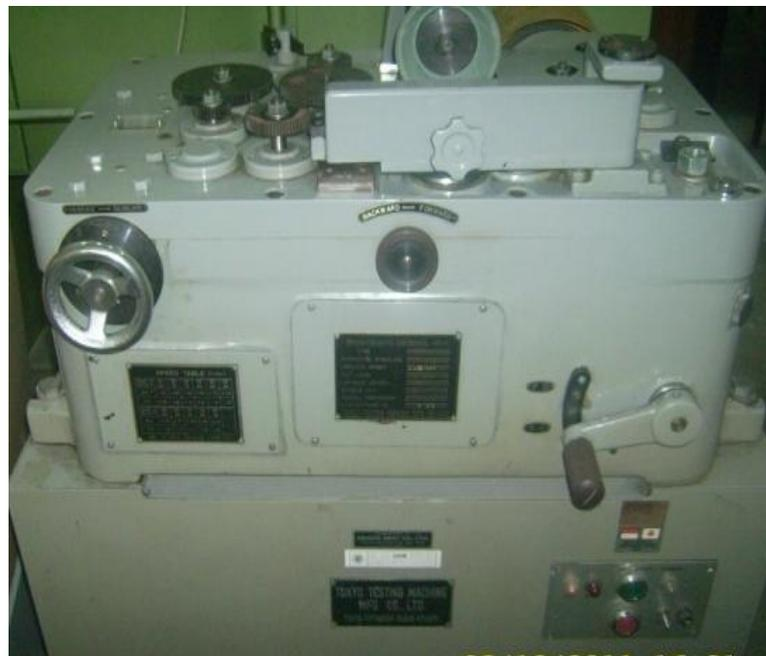
Gambar 3.7 *Ogoshi high speed universal wear testing machine type OAT-U*
