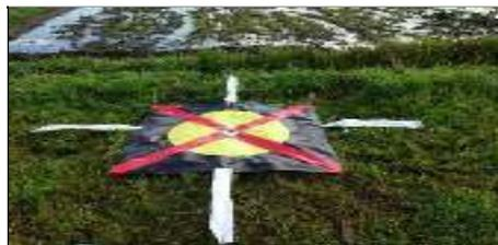
Gambar 2 *Ground control point* (GCP)
