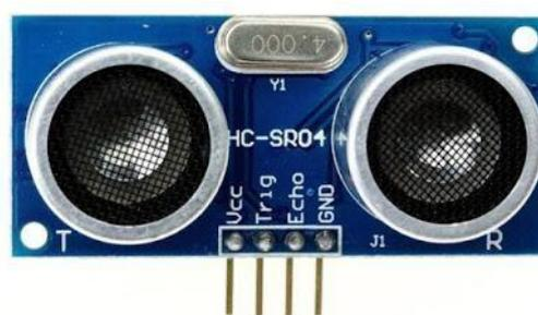
Gambar 2.4 Sensor Ultrasonik HC-SR04
