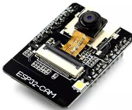
Gambar 2. 8. Modul ESP32-CAM
