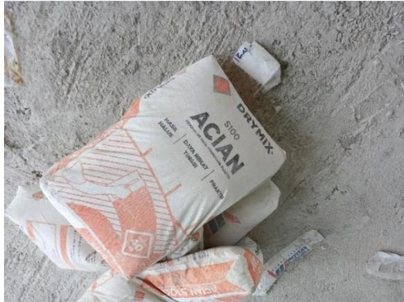
**Gambar 3.23 Mortar acian 50 Kg**
