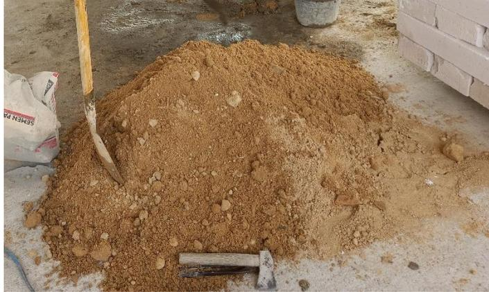
**Gambar 3.16 Agregat halus (Pasir)**
