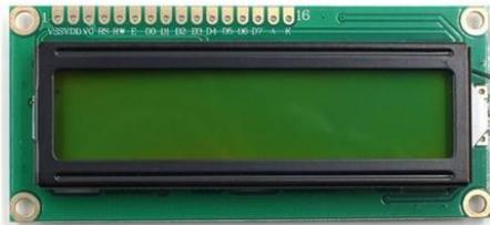
Gambar 9. *Liquid Crystal Display*
