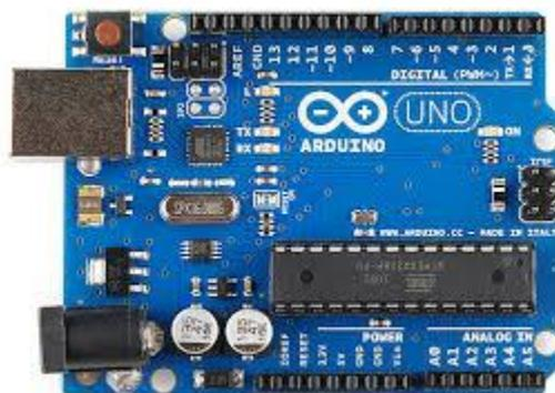
Gambar 6. Arduino USB
