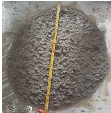
Gambar 10. Pengukuran diameter slump flow .
