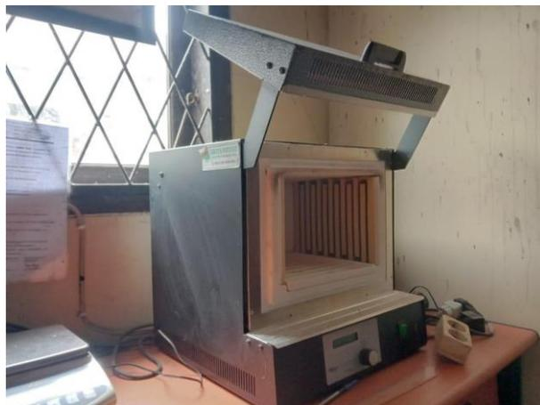
Gambar 5. Alat *furnace* Vulcan D-550
