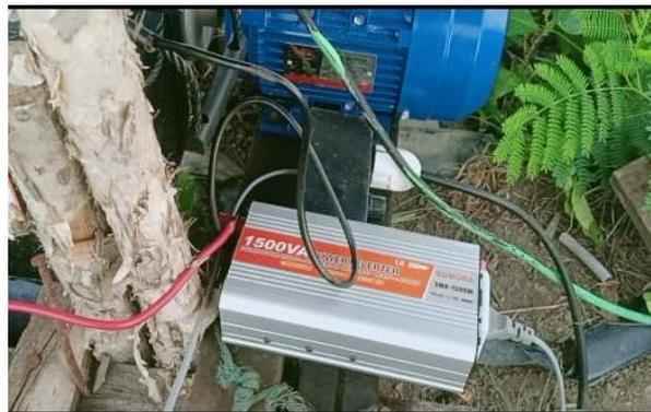
Gambar 3.4 Inverter 12 V to 220. 1200 Watt
