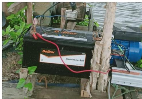
Gambar 3.3 Baterai Delker 12 v 200 Ah
