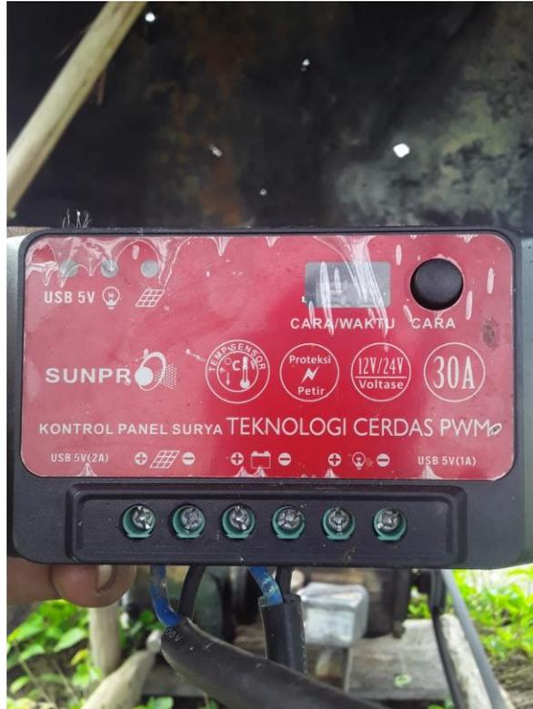
Gambar 3.2 Solar charge controller 30 A
