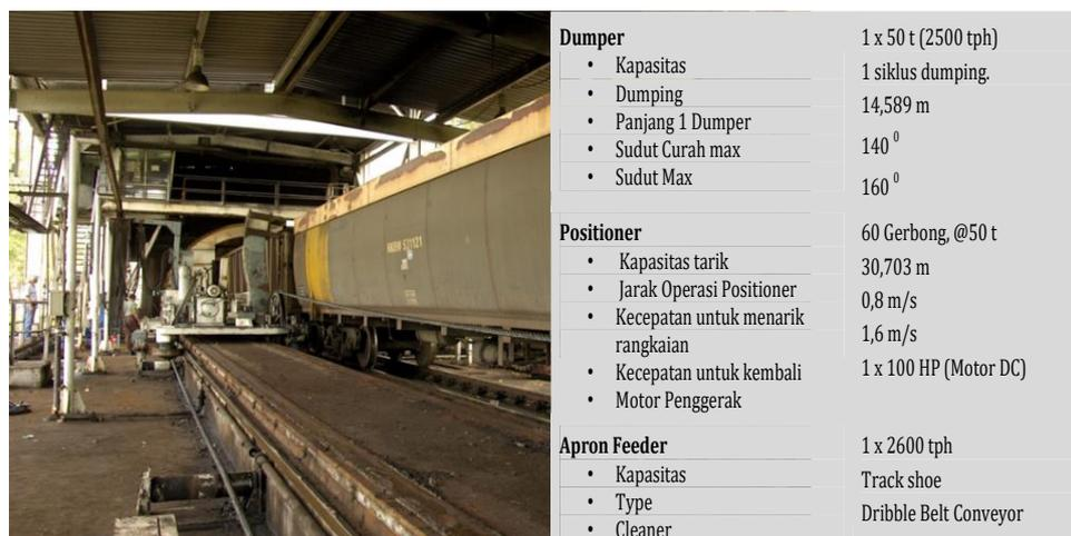
Gambar 5. Rotary Car Dumper (RCD) 2
