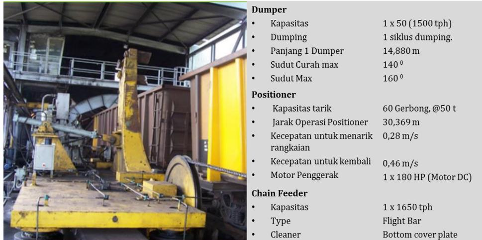
Gambar 4. Rotary Car Dumper (RCD) 1
