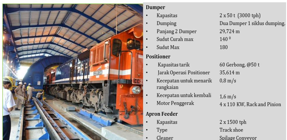
Gambar 6. Rotary Car Dumper (RCD) 3
