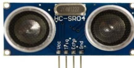
Gambar 2.3 Sensor Ultrasonik tipe (HC-SR04)
