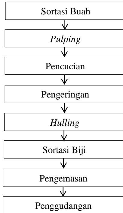
Gambar 2. Diagram Alir Pengolahan Basah ( Wet Process ) Sumber : Mulato (2012)
