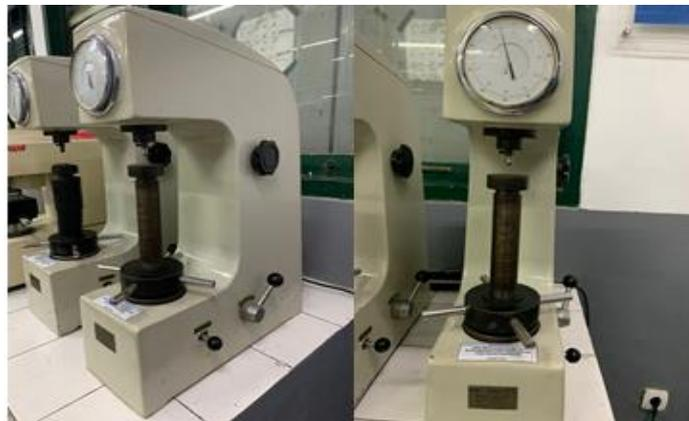
Gambar 10. Alat Uji Kekerasan Rockwell
